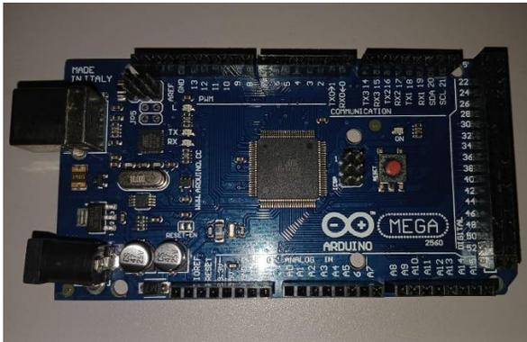
Figura 10: Arduino Mega 2560
